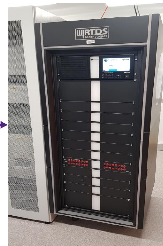
RTDS chassis (NovaCor processor card + GTNETx2 card)
